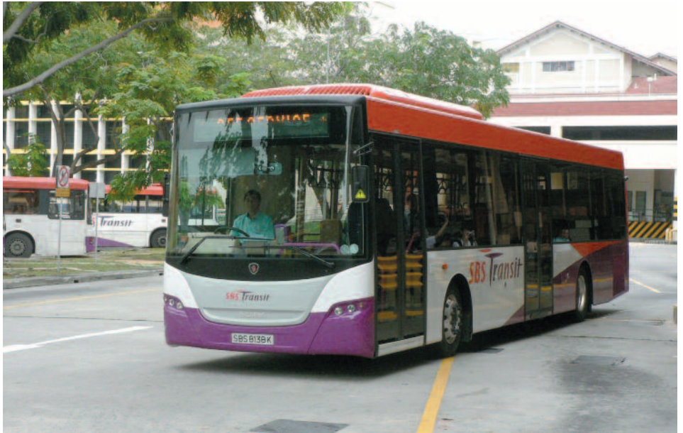
The first 10 Gemilang-bodied Scania K230UB buses for SBS Transit have entered service on routes 100 and 174. Bodywork is supplied in CKD form and assembled by ComfortDelgro Engineering. (Lee IY)
